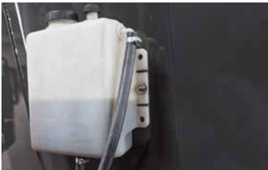
Gearbox oil expansion reservoir
