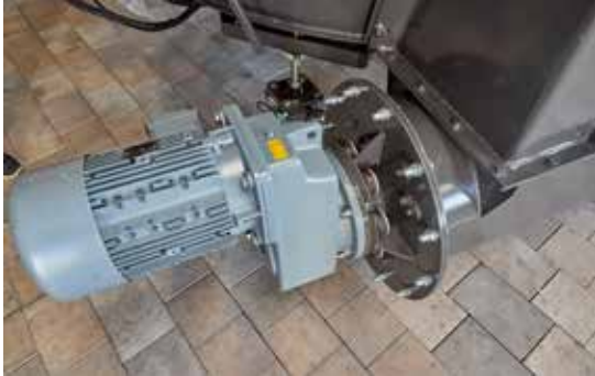
Maintenance-free support: The conveyor auger is supported by the parallel-shaft gearmotor through the gearbox, which runs in an oil bath.
