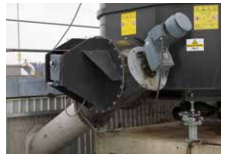
Additional auger for the Rondonmat junction: Provides increased throughput and continuous, consistent material flow; required for feedstock lengths over 50 mm or for materials that are not free-flowing.
