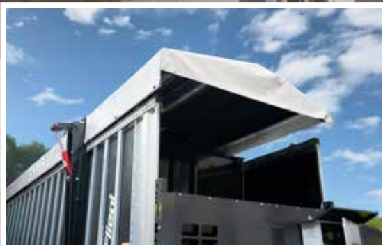
Hydraulically opening roof structure
