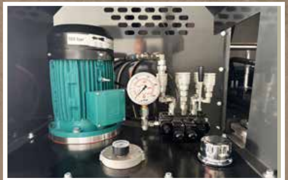
Hydraulic power unit
