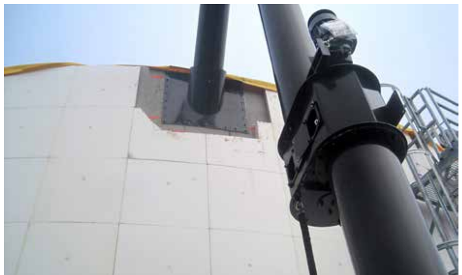
Screw conveyor (casing tube) longer than 7,000 mm with transfer joint.
