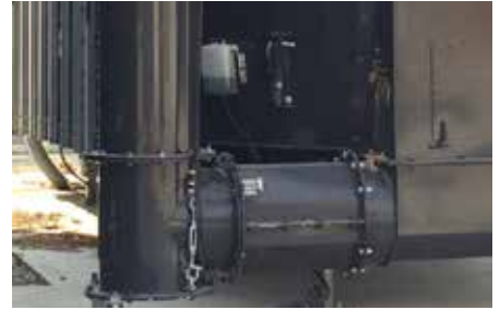
Trough auger with plug joint
