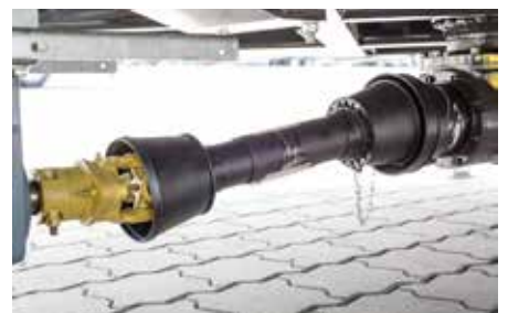
PTO drive with shear bolt
