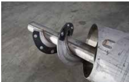
Feeder auger with PE flight
