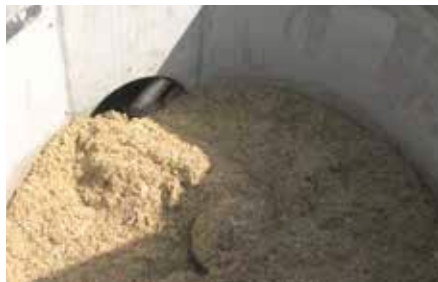
The slow-turning extractor blade has a very low energy requirement.
