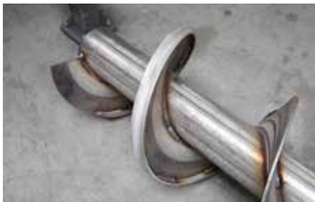
Auger flight with welded-on flat steel
