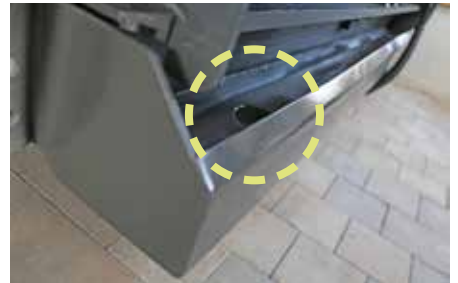
Effluent trough with Ø 100 mm connection
