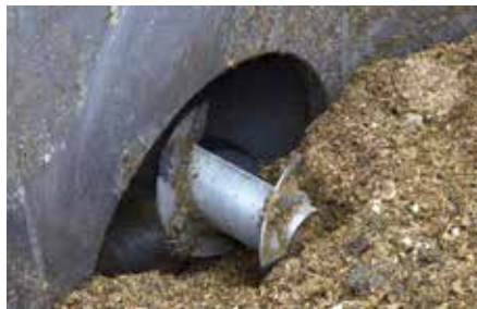
Additional auger for Rondomat joint - required for substrate lengths over 50 mm or for non-free-flowing materials
