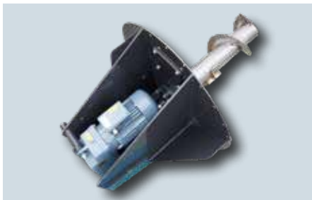
Additional auger for Rondomat joint - required for substrate lengths over 50 mm or for non-free-flowing materials
