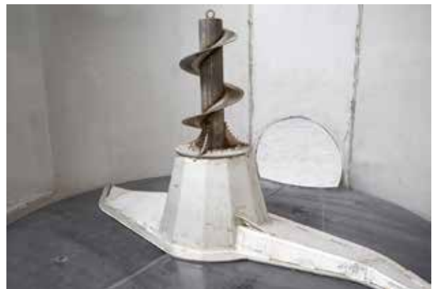
Optional: Stainless steel extractor blade with vertical auger on polyethylene base
