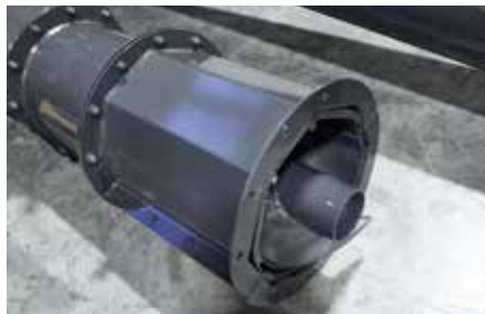
Screw conveyor tube with PE half-shells
