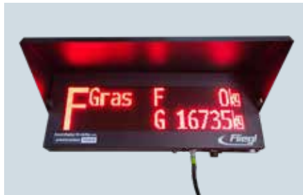
Display: The total weight G and the weight F for the current fill quantity, recorded in ascending order.
